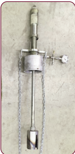
Branch Saddle Assembly Set-up
